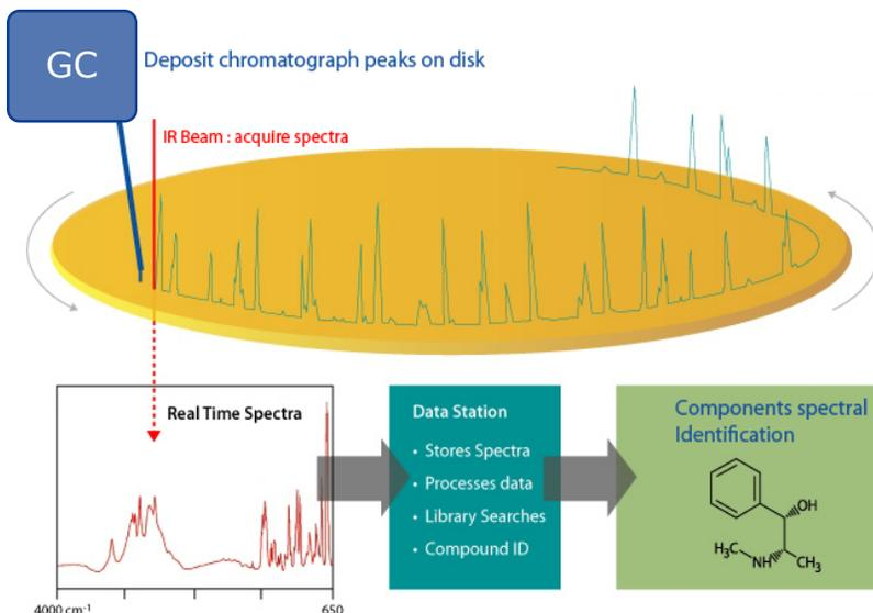
The DiscovIR-GC is a powerful new tool for materials analysis. When connected to the outlet of a GC column, the DiscovIR deposits GC eluents as a continuous track on an infrared transparent substrate. The built-in interferometer simultaneously captures a set of time-ordered infrared spectra from the deposited track. The result is a map of molecular structure of all sample components.
